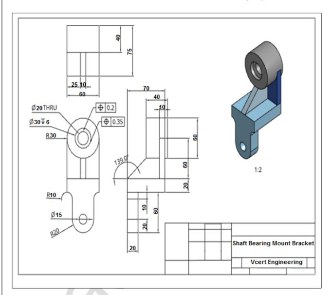
Read the drawing and state in millimetres (mm), the full height, width and depth of the bracket.
