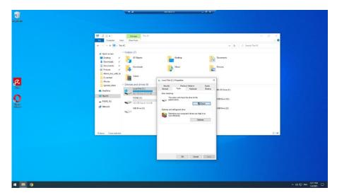
• I run a check on the HDD, which identifies some errors in the file systems. CHKDSK automatically fixes the errors it identified. I also have the computer run a full physical disk check which identifies no issues
