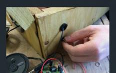
Once my speaker was completed, I had to test the wires to make sure that they went through the holes that I drilled for them, the speaker cable and the switch sit perfectly in the holes that I have made.
