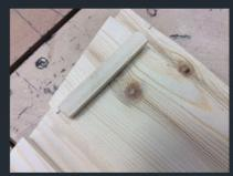
On the two pieces of wood, I have a small strip of wood stuck on, this is to support the cover that will go over the electronics for the speaker. I will make the cover later on and then I will put a speaker in the hole in the back and put the electronics inside the small area.
