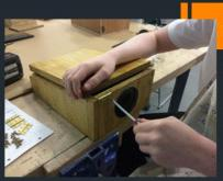
The next part that I added to my product was the lid, and the hinges to make It function like a lid. To put on the hinges I first put them against the wood and put 1 screw into them, this would keep them secure whilst I screw In the other 5 screws. This was also made easy by how soft the wood was, allowing the screw to easily go in by hand.
