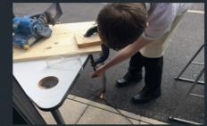
After I had let the glue dry on the wood, I had to sand my wood so it was smooth enough to work with. Before I did the sanding, I had to clamp my wood down onto the table so it was secure and it would not come loose whilst sanding, as it could pose a safety threat. To clamp down the wood I used another small block of wood to put the clamp on as I did not want to damage the wood by clamping it too hard. I used a normal g clamp to keep the wood in place
