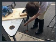
Whenever I used the tools like the sander, I always made sure that it was clamped down and secure so my wood will not come loose and I will not damage it
