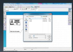
When my product was all put together, I went onto a computer and used 2D design to make a lid for the area where the electronic parts will be. When I have designed it on the computer, I will use the laser cutter to cut it out, black acrylic will be the material that I will use for the lid. To put the design into the laser cutter, I have to export the file as a .DXF file
