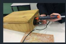
The next thing that I had to do was glue in my speaker, to do this I used a glue gun and applied glue around the edge of the plastic cover and put the speaker on top. This was difficult to do so instead I applied glue to the inside of the plastic instead a stuck the speaker in that way, this was much easier to do and it was also more stable.
