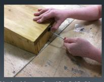
A hook and clasp was the next thing that the lid needed, this was to stop it from opening on its own when tipped and letting the insides fall out, to put on the hook and clasp I simply screwed it in place just like the hinges and it went straight on.
