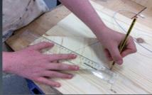
After I sanded the wood, the technician helped me cut the wood into the correct sizes using the table saw. I then had to mark the centre of the wood piece so I could cut out a hole for the speaker
