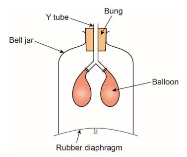
When the rubber diaphragm is pulled down, the volume of the bell jar increases.
