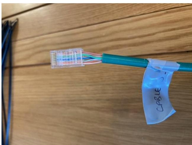
**Cable 4: one RJ45 has been wired 'upside down' but has not been crimped, pulled off, replaced RJ45 and crimped. Then labelled 'Cable 4'**
