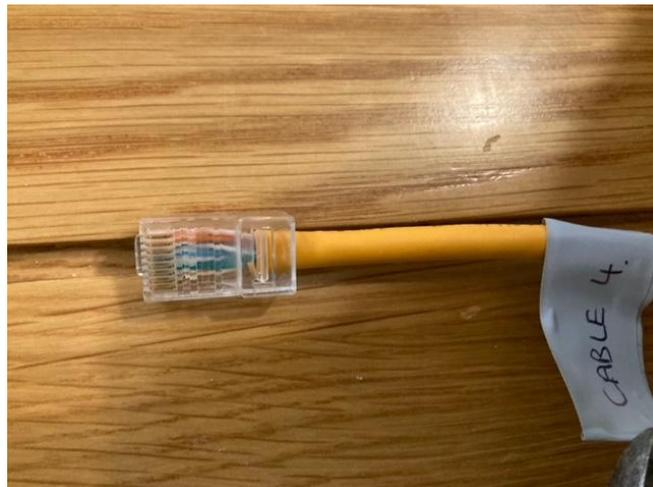
**Cable 5: the wires within one end of the cable do not reach the copper pins within the RJ45, this was removed and replaced correctly. Then this was labelled 'Cable 5'**
