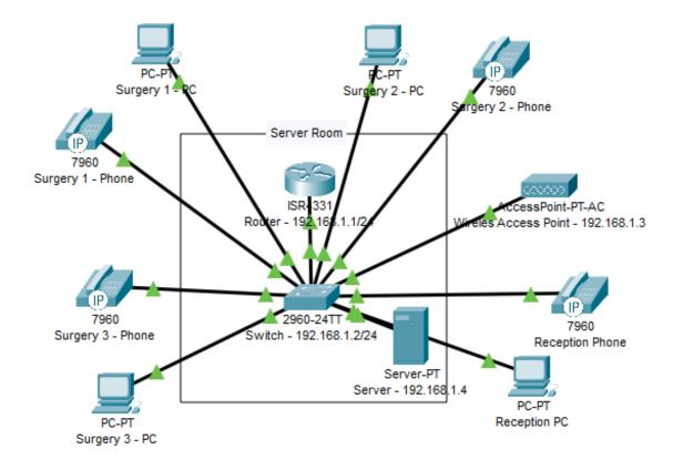
The server is configured as a DHCP server to complete DHCP requests made by devices on the network. All devices communicate via the switch unless access to resources outside of the network are required, then the router is utilised.
